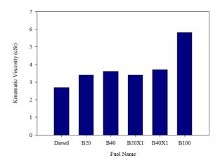
Figure 3 Kinematic Viscosity of Various Fuels Kinematic viscosity for pure Mahua biodiesel and B20 are 5.8 cSt and 3.4 cSt respectively, whereas for diesel kinematic viscosity measured is 2.7 cSt. This is shown in figure 3 Mahua bio- diesel has 1.9 times higher kinematic viscosity compared to diesel. Density of Mahua bio-diesel is 0.824 g/cc where as diesel has density of 0.818 g/cc. Due to higher density of Mahua bio-diesel, specific fuel consumption will be less than diesel
