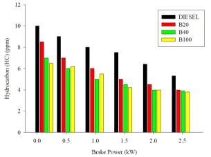
Figure 8 Variations in Hydrocarbon Emission with Brake Power And Bio-diesel Percentage in blend
