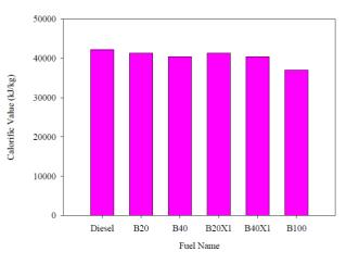
Figure 2 Calorific Values of Various Fuels
