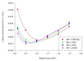
Figure 7 Variations in Carbon Monoxide Emission with Brake Power And Bio-diesel Percentage in blend Hydrocarbon
