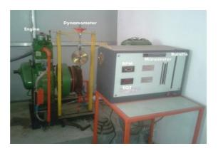
Table 3 Engine Specification Make Kirloskar General details single cylinder four stroke diesel engine Number of cylinders one Rated speed 1500 RPM BHP 5 KW SFC 3.7 Bore 110mm Orifice Dia 20 mm
